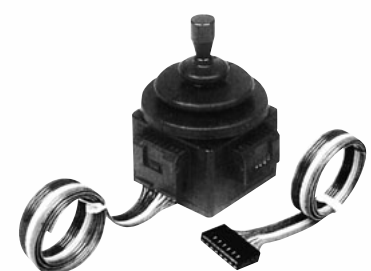
40JEK-YQ-07R2G (4 bit gray code) 40JEK-YQ-08R2G (4 bit binary code) 40JEK-YQ-075R2G (5 bit gray code) (2-dimensional coordinate type) with dust-proof rubber cover)
